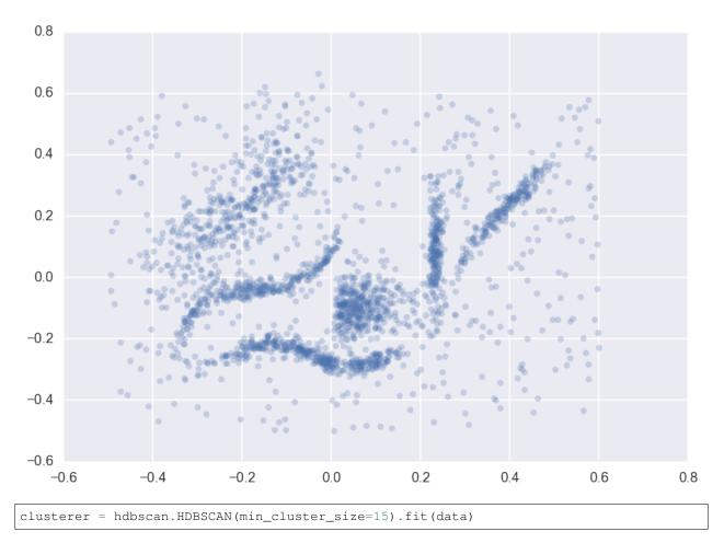
The clusterer object now has an attribute (computed when first accessed) called outlier\_scores\_. This provides a numpy array with a value for each sample in the original dataset that was fit with the clusterer. The higher the score, the more likely the point is to be an outlier. In practice it is often best to look at the distributions of outlier scores.
