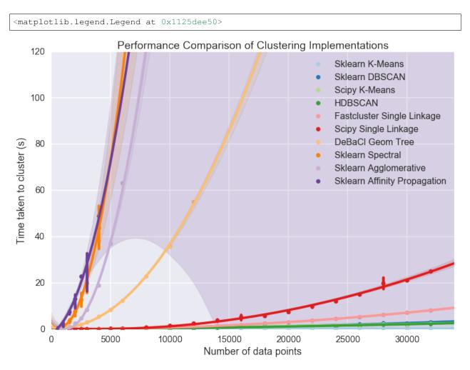
A few features stand out. First of all there appear to be essentially two classes of implementation, with DeBaCl being an odd case that falls in the middle. The fast implementations tend to be implementations of single linkage agglomerative clustering, K-means, and DBSCAN. The slow cases are largely from sklearn and include agglomerative clustering (in this case using Ward instead of single linkage).
