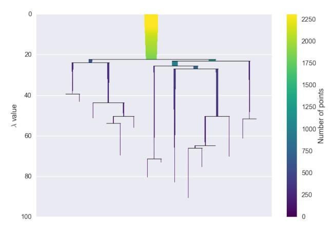
We can now see the hierarchy as a dendrogram, the width (and color) of each branch representing the number of points in the cluster at that level. If we wish to know which branches were selected by the HDBSCAN\* algorithm we can pass select\_clusters=True. You can even pass a selection palette to color the selections according to the cluster labelling.
