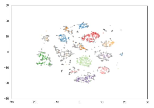
Increasing the min\_cluster\_size to 30 reduces the number of clusters, merging some together. This is a result of HDBSCAN\* reoptimizing which flat clustering provides greater stability under a slightly different notion of what constitutes a cluster.
