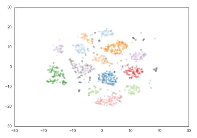
Now most points are clustered, and there are much fewer noise points. Steadily increasing min\_samples will, as we saw in the examples above, make the clustering progressively more conservative, culminating in the example above where min\_samples was set to 60 and we had only two clusters with most points declared as noise.
