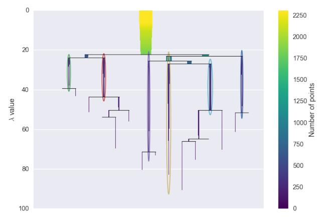
From this we can see, for example, that the yellow cluster, at the center of the plot, forms early (breaking off from the pale blue and purple clusters) and persists for a long time. By comparison the green cluster, which also forms early, quickly breaks apart and then vanishes altogether (shattering into clusters all smaller than the min\_cluster\_size of 15).
